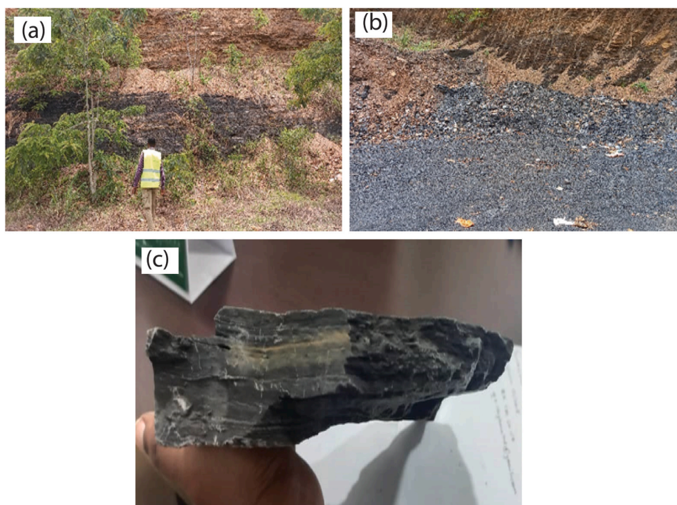
Fig. 2. (a) Field photos showing a cliff face of a darker shales outcrop. (b) Broken black shales showing depth extension as a result of excavation (c) Shale show typical laminated feature.
