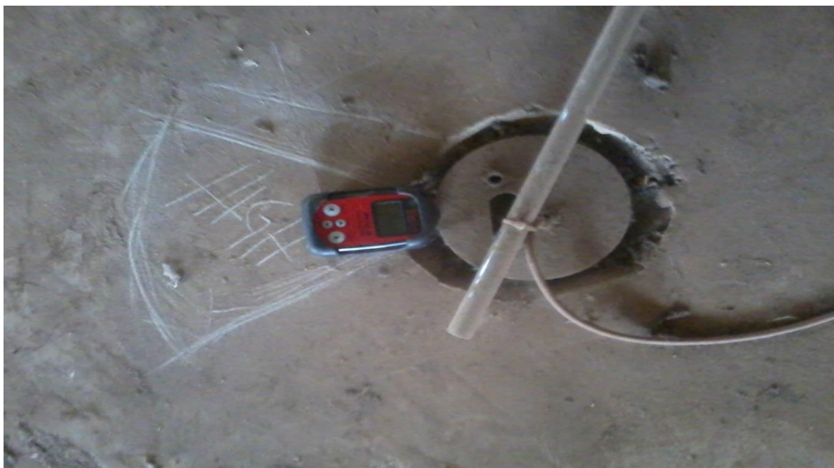
Plate 4.2 Gamma Survey Meter recording value at “high point” of roof plug3
