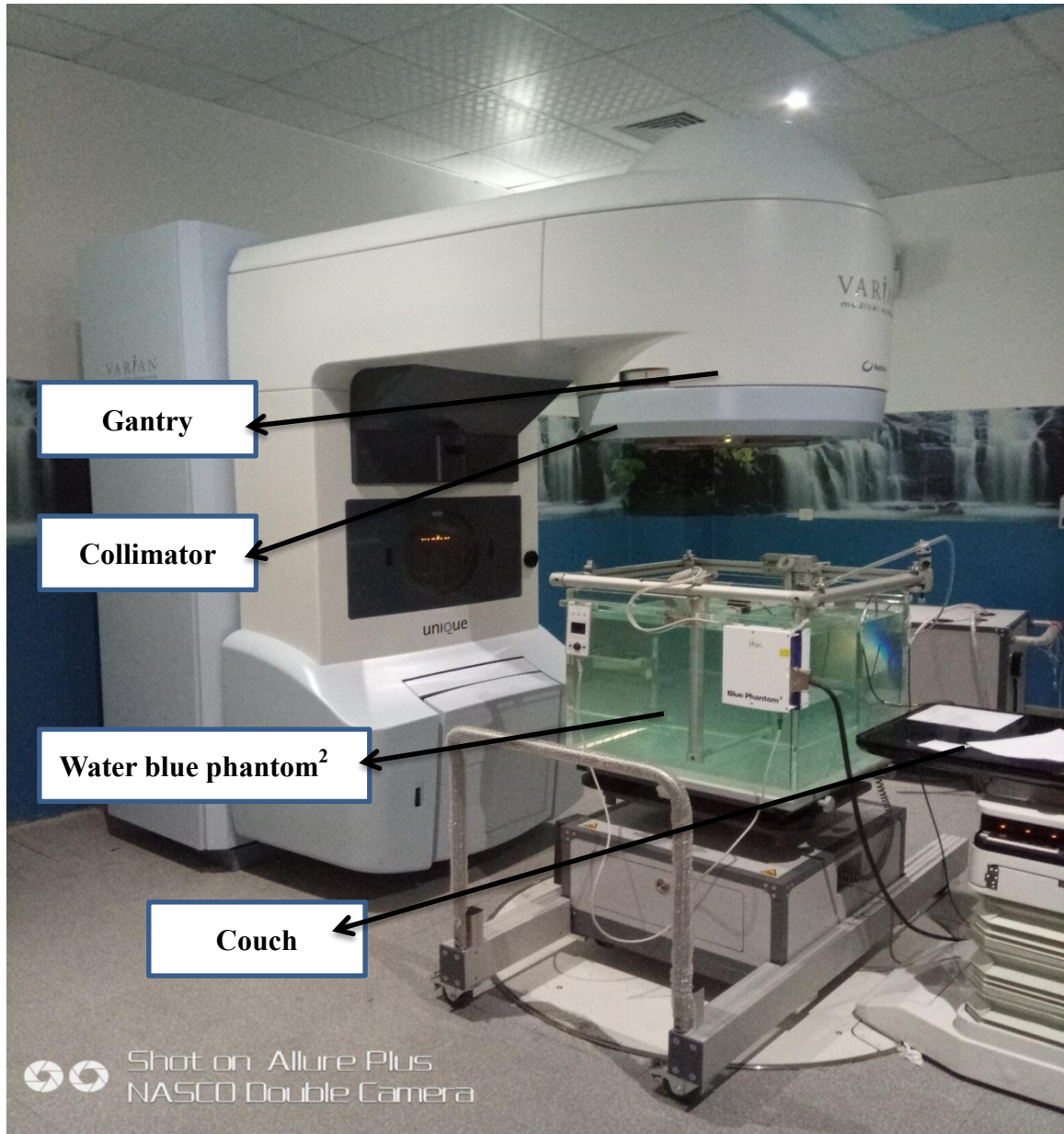
Figure 3. 3: Varian Unique Performance medical system linear accelerator with motorized water phantom set up for beam data acquisition.
