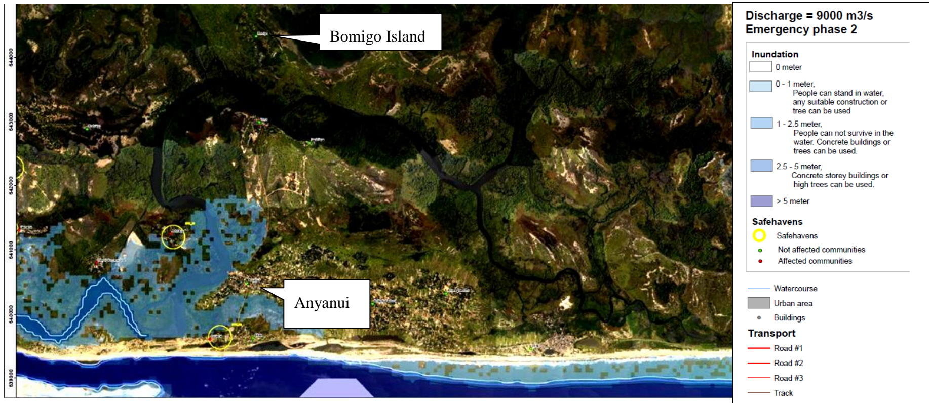
Figure 4.4 Inundation map of study communities in Keta Municipal at 9000 m 3 /s discharge rate
