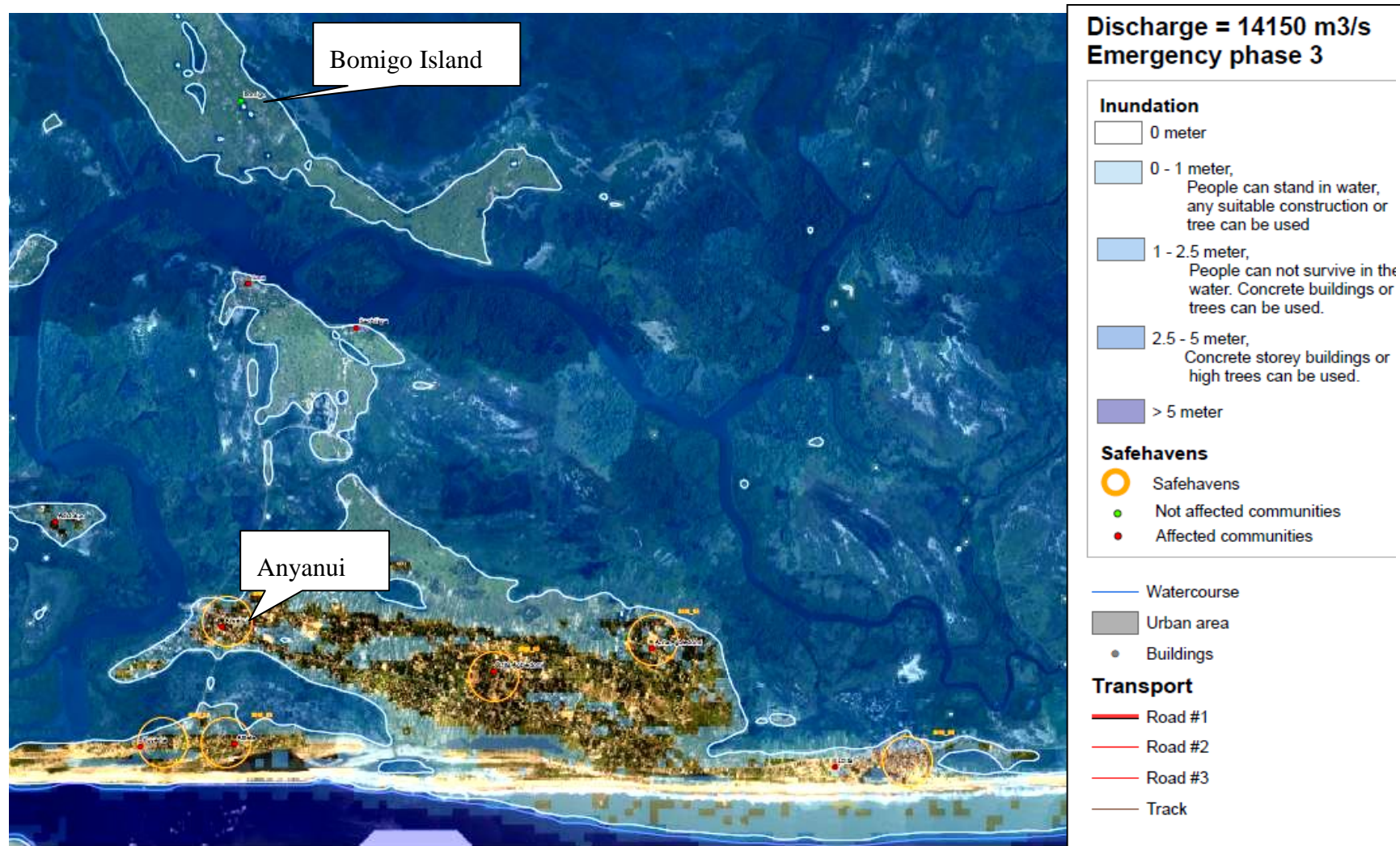
Figure 4.6 Inundation map of study communities in Keta Municipal at 14150 m 3 /s discharge rate
