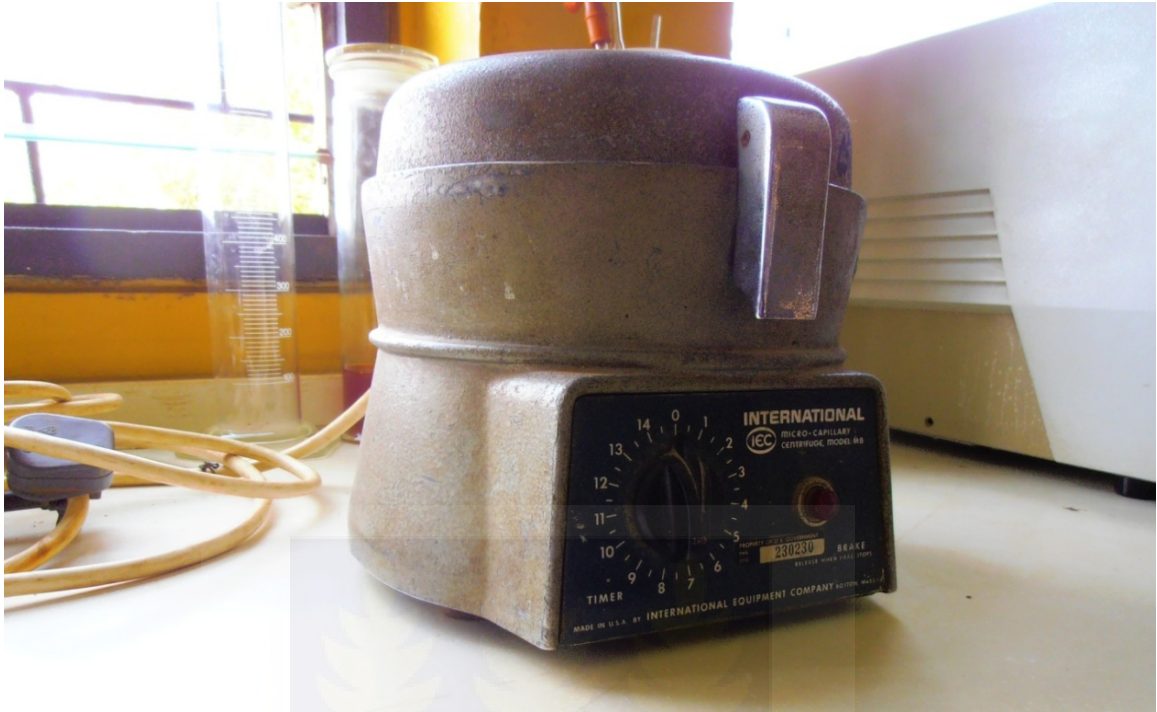
Plate 3.3: Micro-capillary centrifuge (Model MB, International Equipment Company, Boston, U.S.A)
