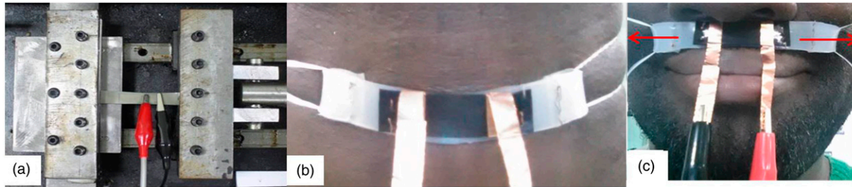
Figure 1. Experimental set-up for some applications: (a) dynamic cyclic test (b) sensor placed at the throat, and (c) sensor placed in-between upper lip and the nose.
