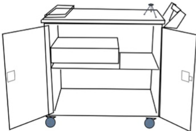
Fig. 2 The system's cabinet showing two padded shelves
