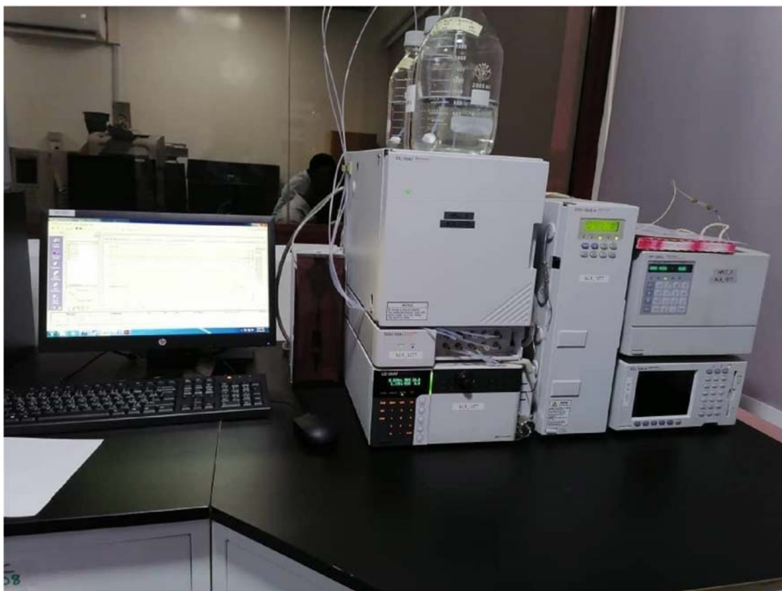
Plate 1: Shimadzu HPLC-FLD system (Kyoto, Japan), Autosampler (SIL-10AF) at Quality Control Company (QCC) of COCOBOD, Tema Laboratory (x1/15).
