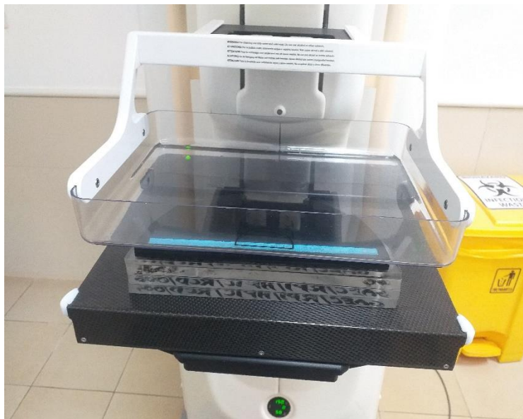
Figure 3.14: Set – up for spatial resolution with TORMAS phantom (Field Work)
