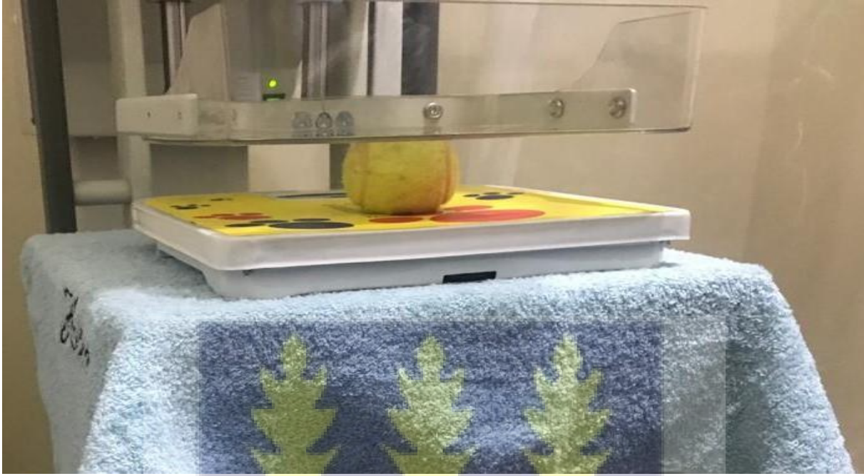
Figure 3.9: Set-up for compression force (Field Work)
