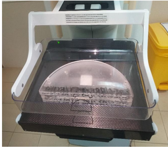
Figure 3.13: Set-up of the PMMA and the sandwiched aluminum filter (Field Work)
