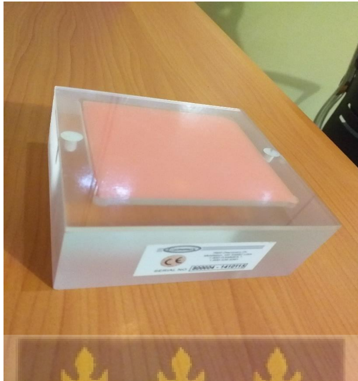
Figure 3.4: The American College of Radiologist Mammography Accreditation Phantom (ACR MAP) - (Field Work)
