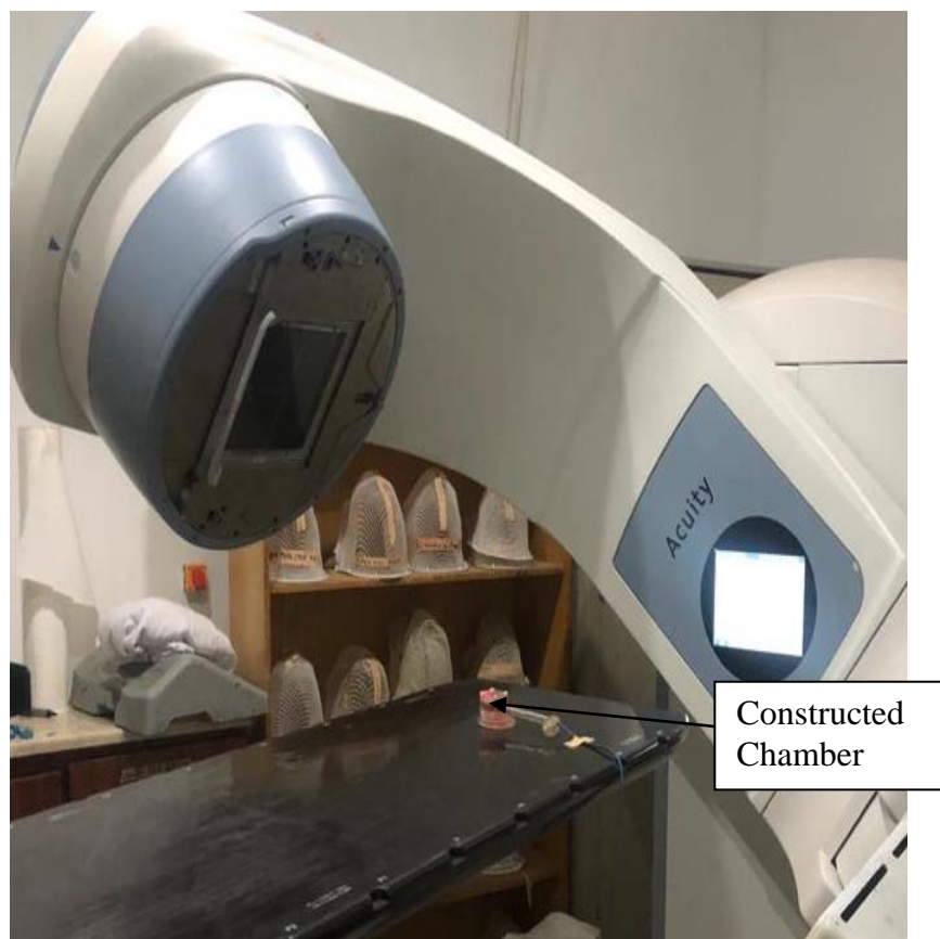
Figure 3.11: Set- up for the determination of angular dependency of the constructed chamber.
