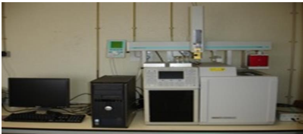
Plate 4.4: GC Varian CP-3800 for organochlorine pesticide Quantification
