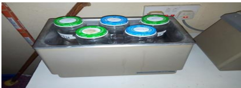
Plate 4.2: Extracts in a Bransonic 220 high-frequency ultrasonic bath
