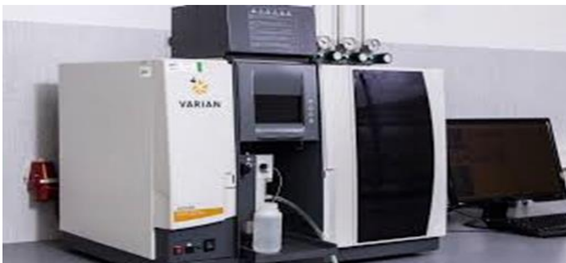
Plate 4.5: Varian AA 240FS- Atomic Absorption Spectrometer
