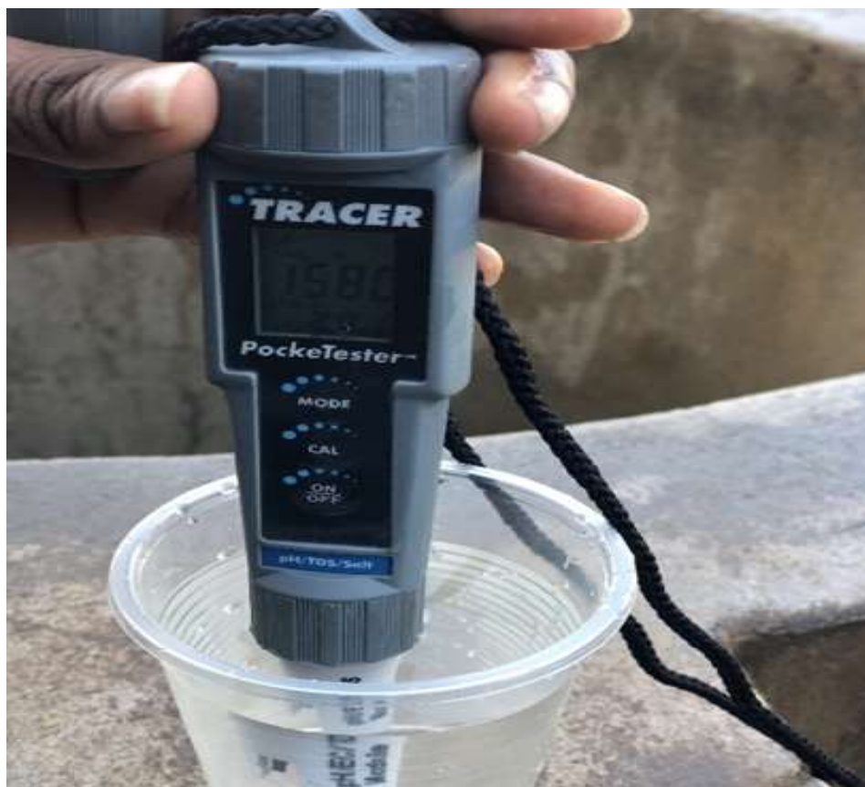
Figure 3.4: Measurement of physical parameters with LaMotte Tracer PockeTester meter
