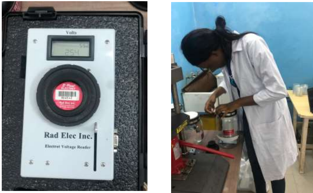
Figure 3.5: An E-perm detector used to measure Radon
