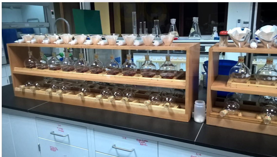
Figure 3.5: Filtration set up for pesticide residues extraction
