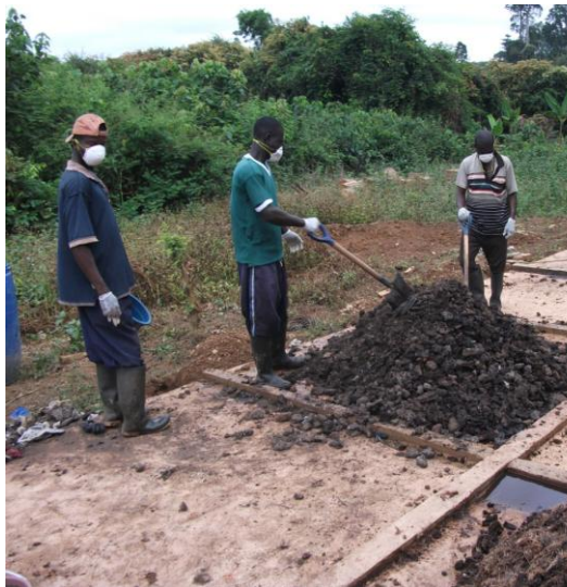
Plate 3.8: Mixing and building of compost windrows
