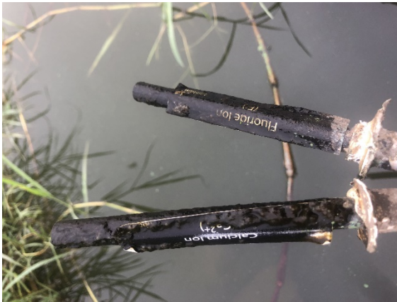
Figure 6. 31 Biofouling (fluoride and calcium sensors)
