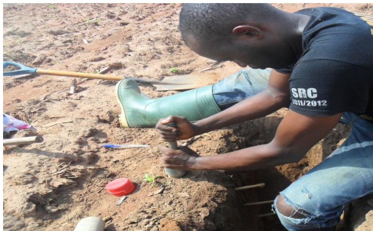
Figure 8: Soil sampling on the field
