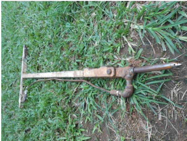
Figure 4.1c. The ethylene gas injector
