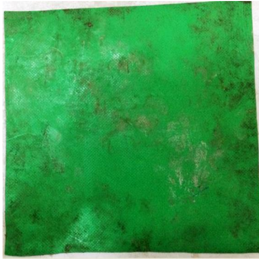
Figure 2. 6 Plastic Sheet for curing of mortar and concrete cubes
