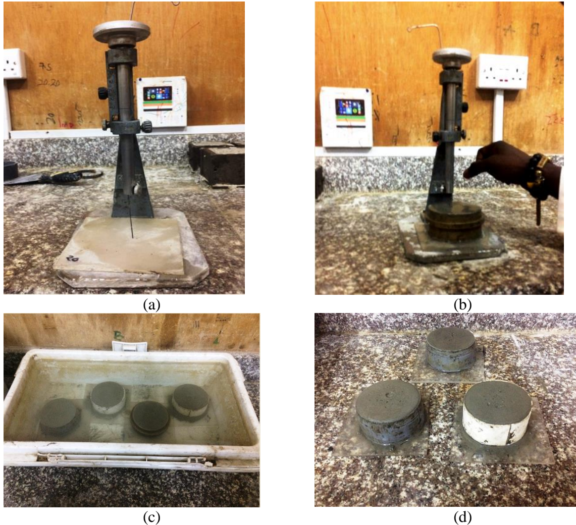
Figure 3. 4 Procedure for determining initial setting time
