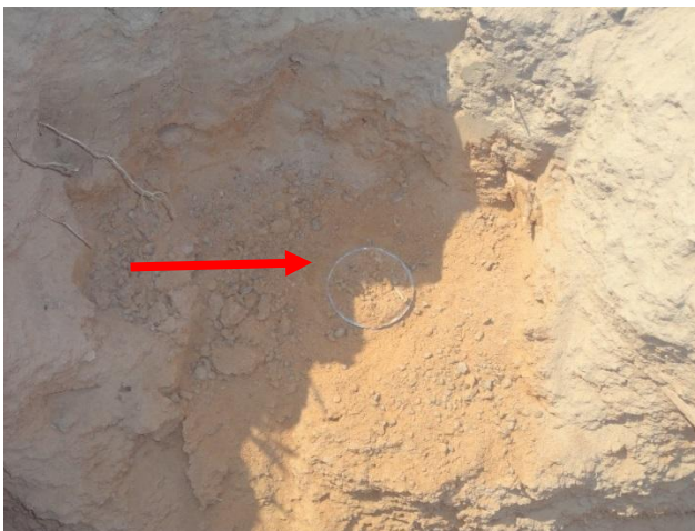
Figure 3.16. Taking undisturbed core samples from soil profile
