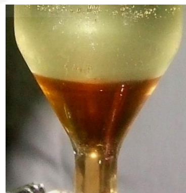
Fig. 3.8: The aqueous and organic layers obtained after addition of dithizone in CHCl_3 solution. The pink colour of the CHCl_3 layer is due to the Pb-dithizonate present.
