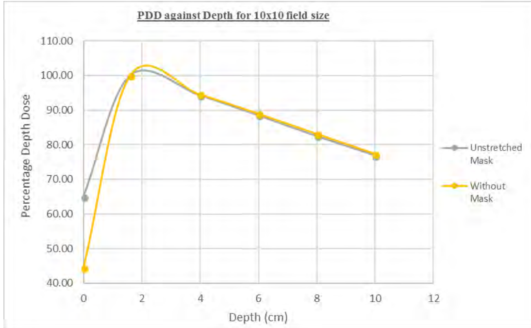
Figure 4. 5: A graph of PDD against Depth for a 10x10 field size with an unstretched mask and without a mask.
