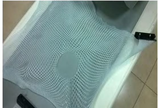
Figure 2. 3: A stretched thermoplastic mask to be used on the solid water phantom
