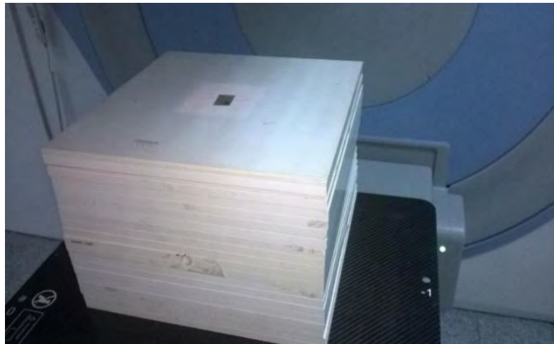
Figure 3. 16: Positioning of the film set A, B, and C at the surface of the phantom, at the d_{\text{max}} of 1.6 cm for the 6 MV photon beam, and at a depth of 10 cm respectively
