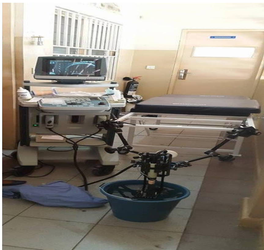
Plate 3.10: The set up for the template grid alignment test.
