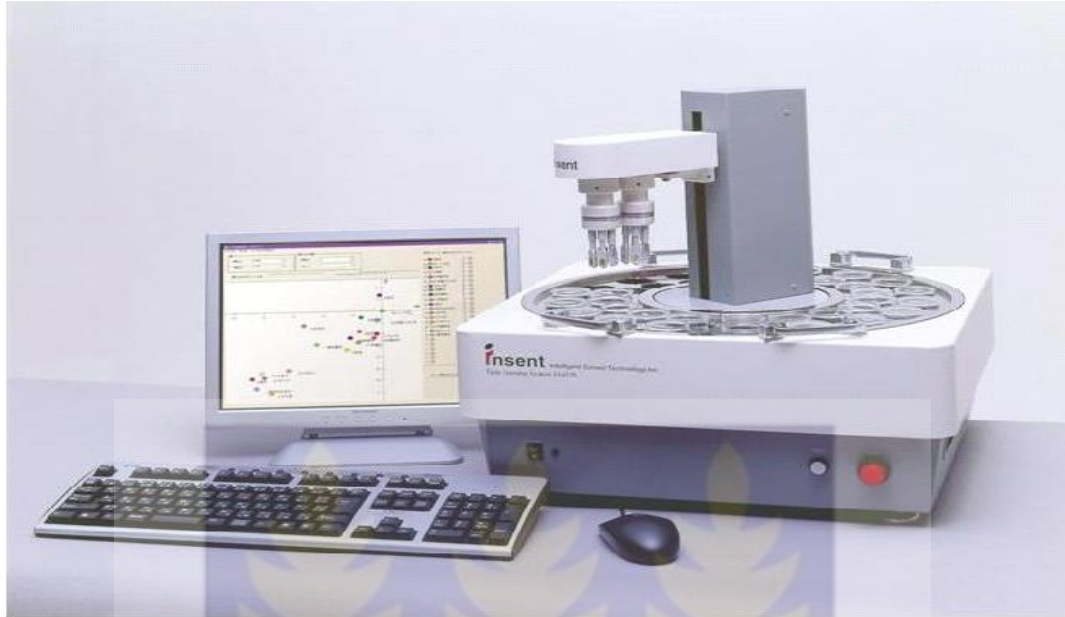
Figure 5A Simple Electronic Tongue (Taste-Sensing System SA 402B)
