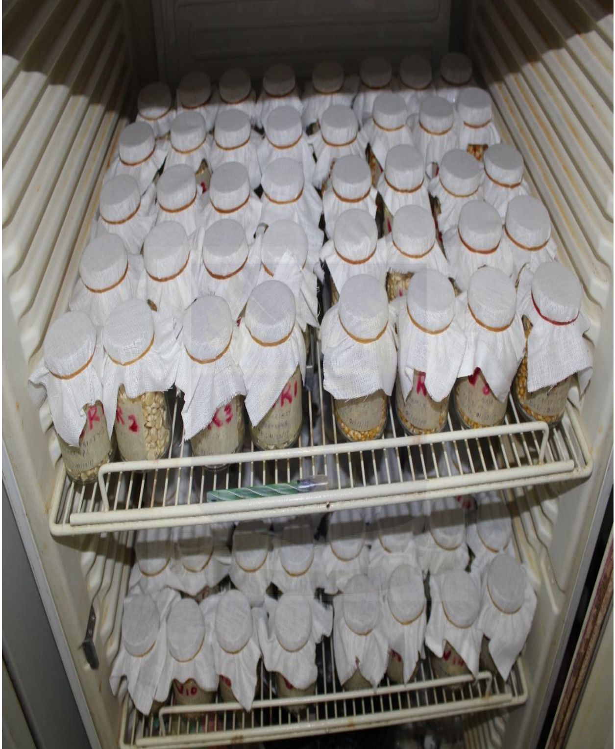
Plate 2: Experimental set up of 18 maize varieties in Rubarth Apparate GmbH RUMED test chamber.
