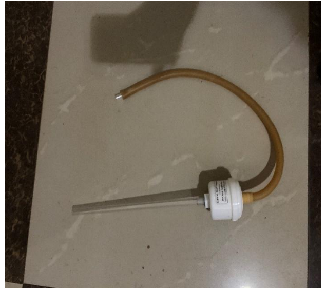
Plate 4. Mouth aspirator for mosquito collection
