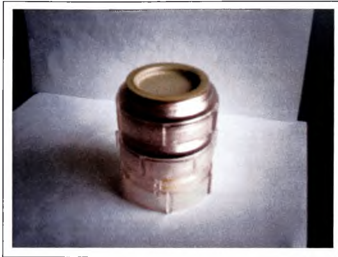
FIGURE 4-2 TWO STAGE STACK FILTER CASSETTE UNIT (SFU) LOADED WITH FILTERS AND CAPPED
