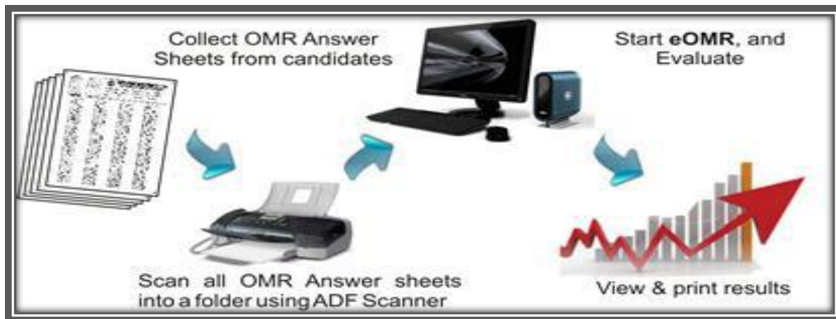
Figure 2: Optical Mark Registration Process
