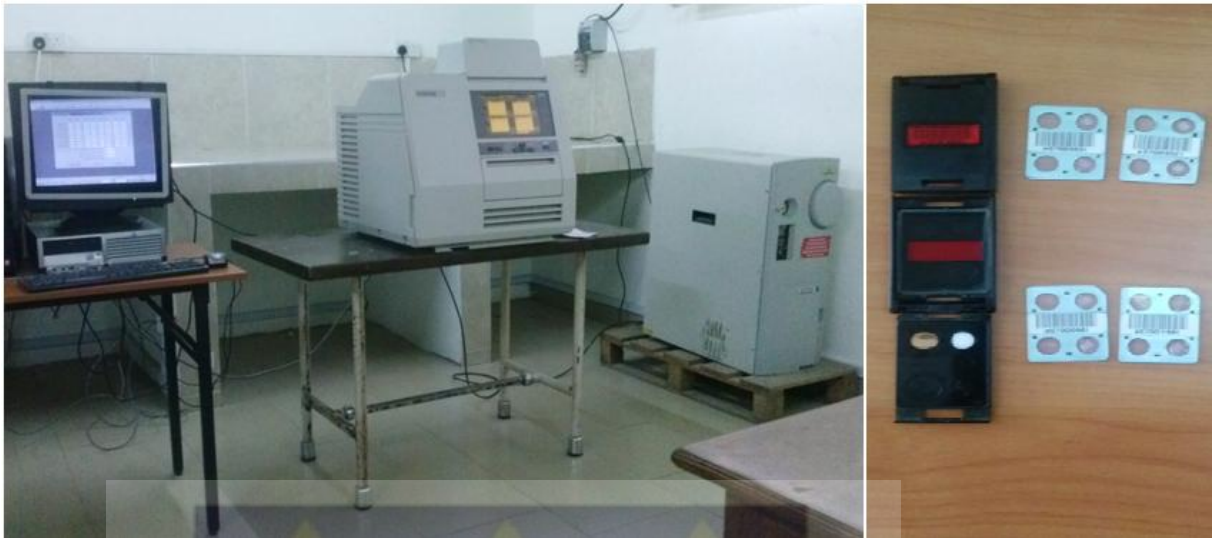
Figure 3.1: Harshaw 6600 system of the dosimetry service of Ghana. Here are presented the dosimeters, the gas generator, the reader and the personal computer of this dosimetry system.
