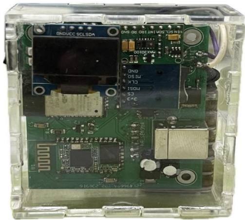
Figure 34. Front view of the electronics enclosure of the Holter Monitor (Researcher's own construct,
