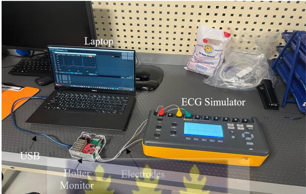
Figure 42. This figure shows a set-up of the system simulation with the Holter Monitor connected to the laptop via USB cable and the electrodes connected to the corresponding pins on the ECG Simulator
