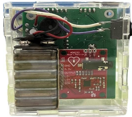
Figure 33. The back view of the electronic enclosure of the Holter Monitor (Researcher's own construct, 2023).
