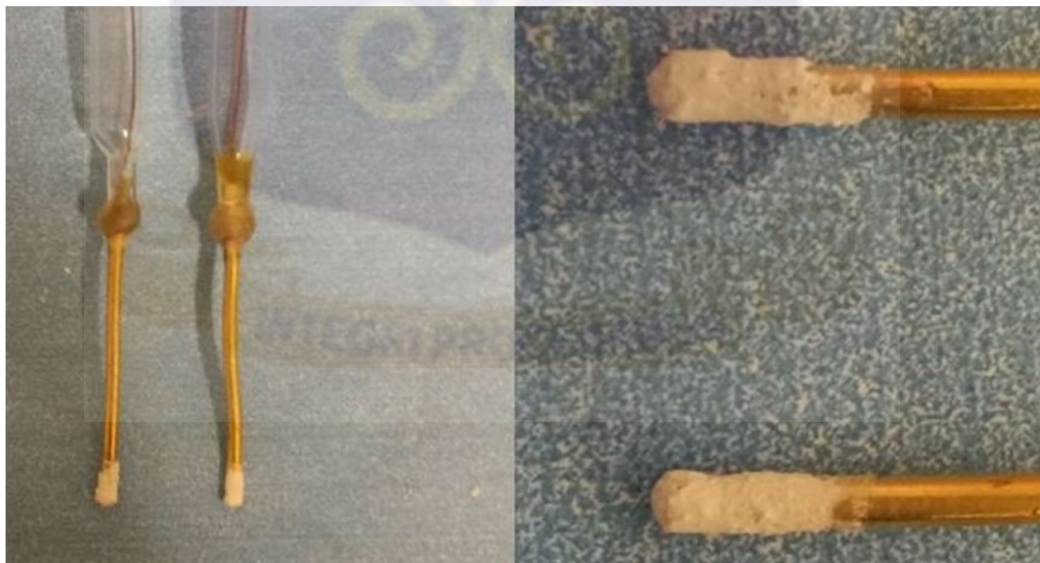
Figure 12: Thin layer of zeolite deposited on the gold electrode active zone after dehydration.
