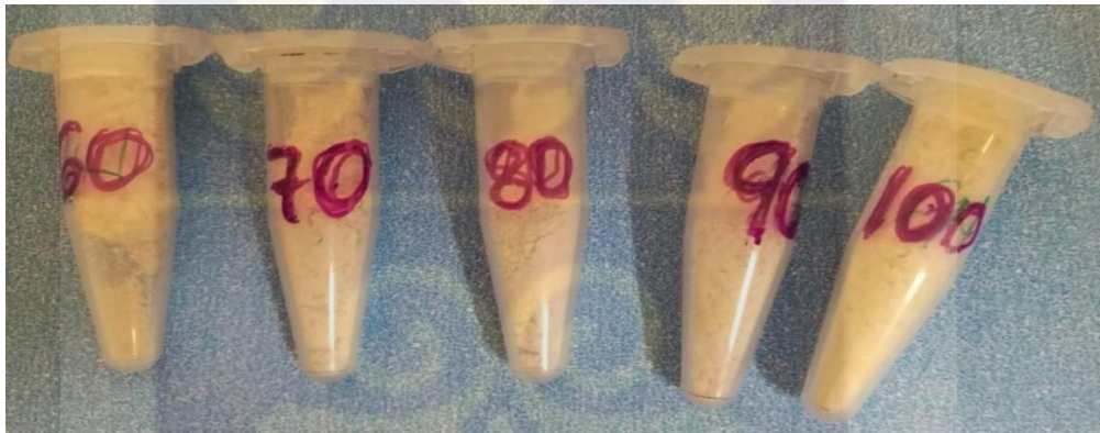
Figure 7: (a) Synthesized zeolites at different crystallization temperatures, (b) Packaged crystalline material for biophysical analysis.
