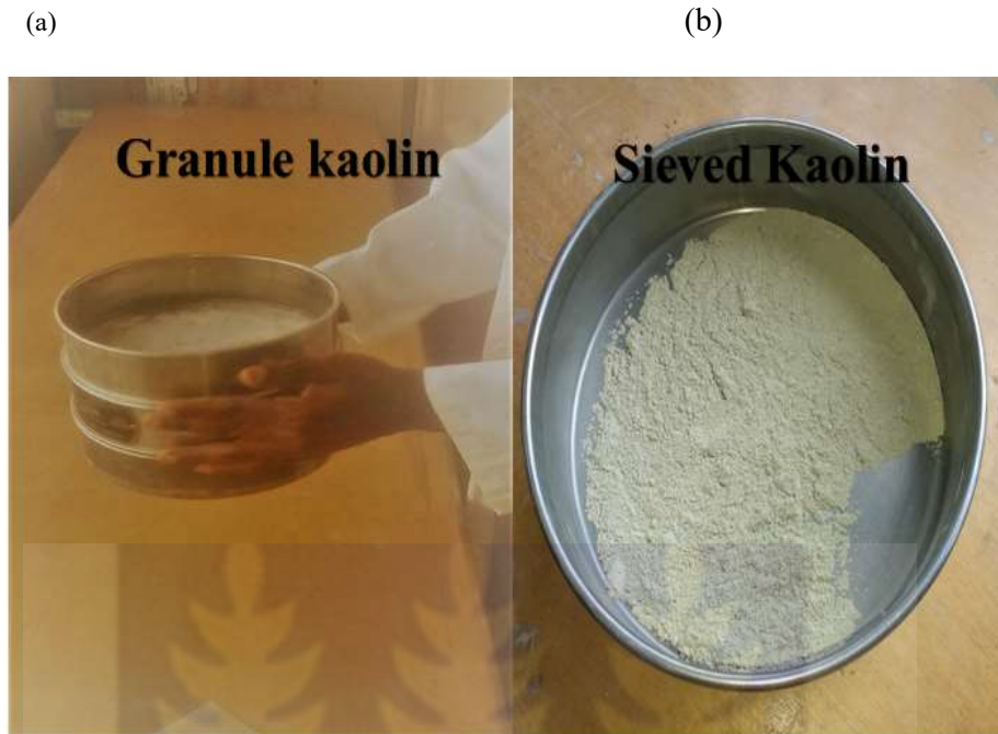
Figure 3: (a) Depicts sieving of grounded kaolin, (b) Fine grains of kaolin sieved with 63 \mu\text{m} .
