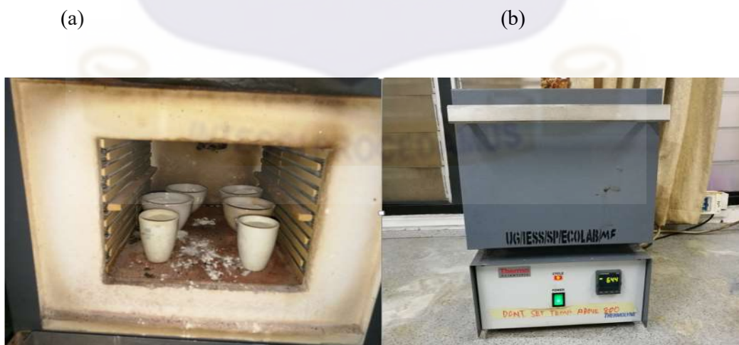
Figure 4: (a) Shows crucibles filled with kaolin and placed in a furnace, (b) shows the furnace used to heat the kaolin to the desired temperature to obtain metakaolin.
