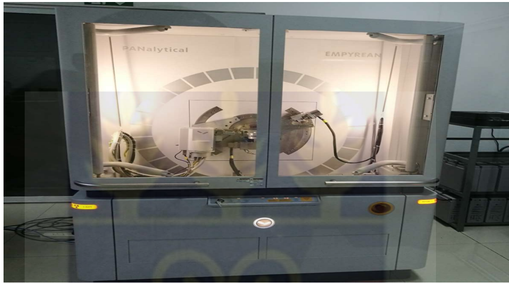
Figure 8: XRD equipment used for diffraction analysis at the University of Ghana, Department of Physics.
