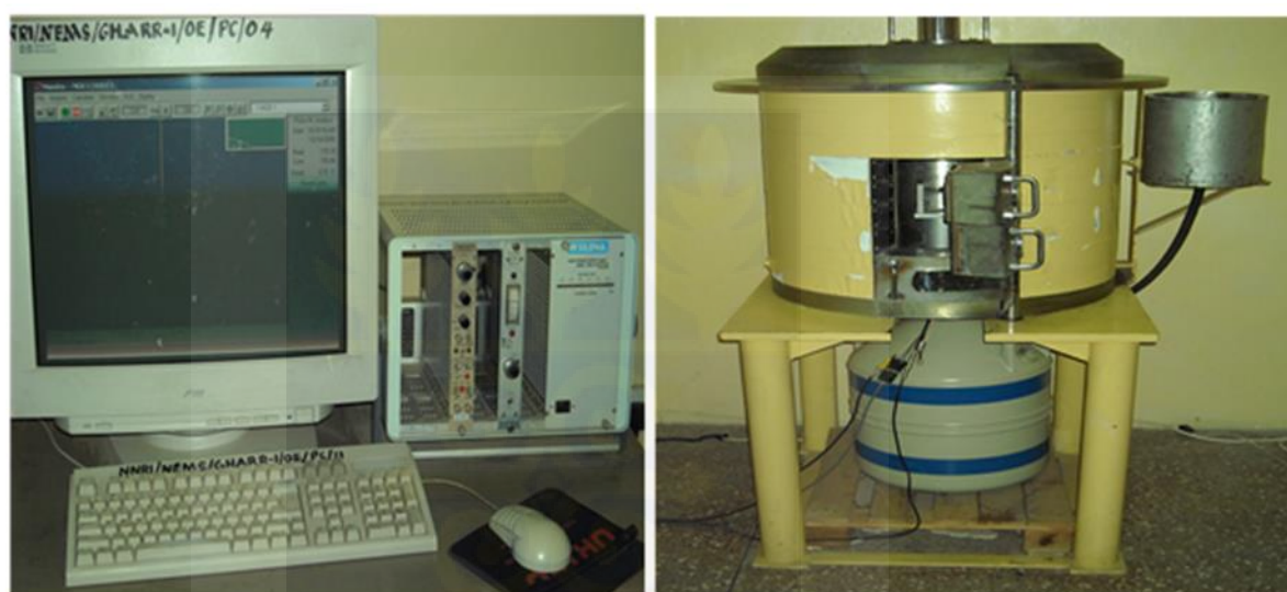
Figure 4.1 A PC based gamma-ray spectroscopy system coupled to high germanium (HPGe) \gamma -ray detector
