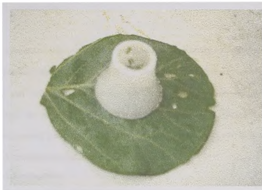
Plate 5. Larvae immersion bioassay set up. Plastic cup “holy communion cup” (about 2.74cm depth, bottom and top radii are 3.42cm and 2cm respectively). With net-like material at the bottom and an open top end.
