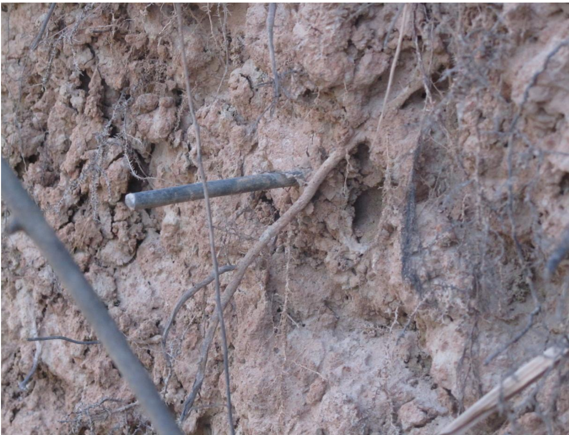
Plate.5.1: Erosion Pin at the bank of the Birim River at Akim Oda
