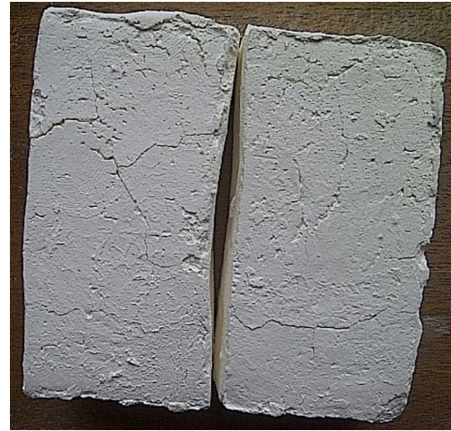
Fig. 16. Porous ceramic with HDPE as pore former showing micro cracks.
