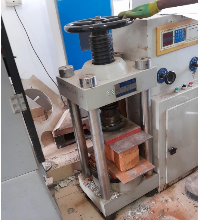
Figure 3. 8 Compressive Strength test
