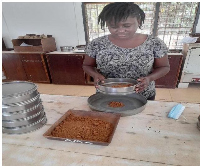
Figure 3. 4 Particle sieve analysis
