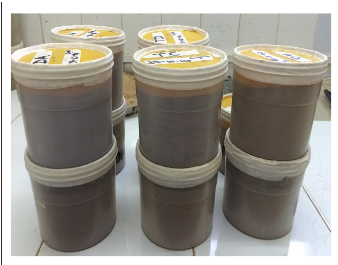
Figure 3.7: Sealed Marinelli beakers containing soil samples.
