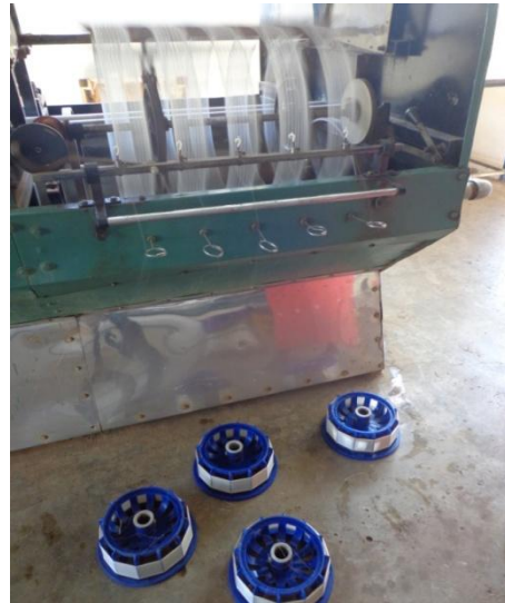
Plate 2.4 Re - reeling onto standard reels.
