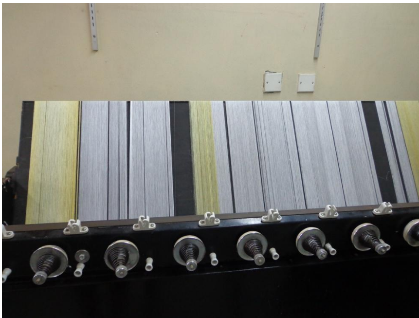
Plate 3.10 A seriplane for testing cleanliness and neatness of raw silk in the silk quality laboratory at ICIPE, Nairobi.
