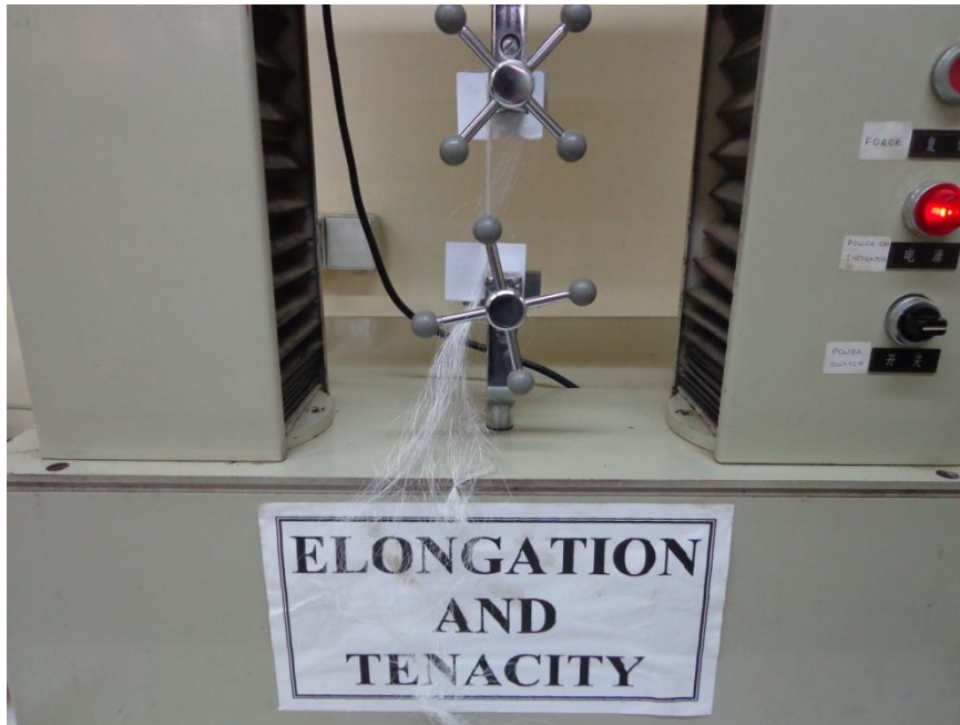
Plate 3.9 A serigraph for testing the tenacity and elongation of raw silk yarns at the silk quality laboratory at ICIPE, Kenya.
