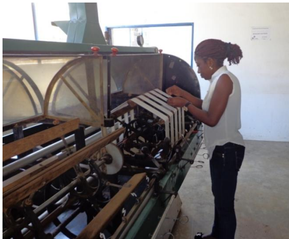
Plate 2.5 Lacing of silk skeins on standard reels at the silk processing laboratory, ICIPE, Nairobi.
