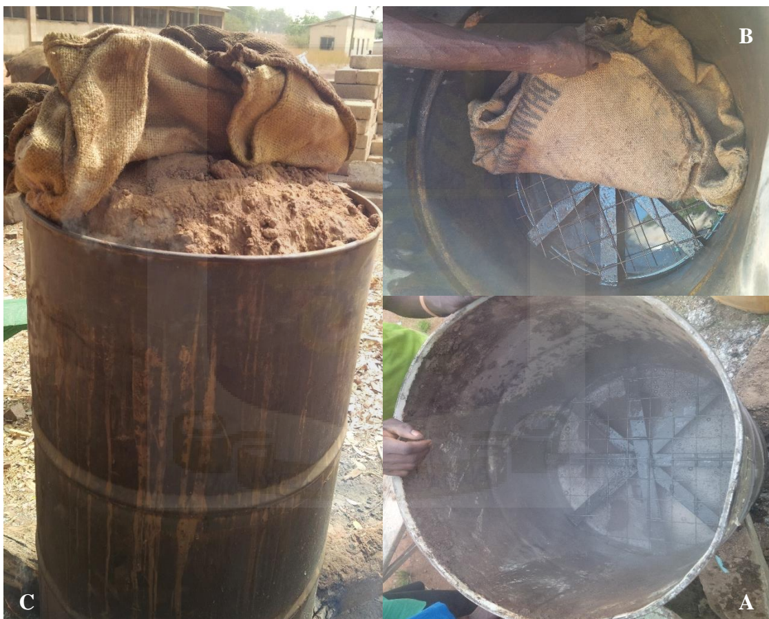
Plate 3.1 Photograph of the drum approach, Drum filled with water to the mesh level (A), Drum with jute sack sealed/place on the mesh (B), Drum filled with soil mixture for initiation of sterilization (C)
