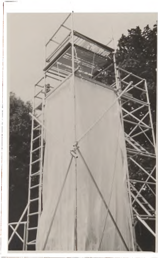
PLATE 6. Raintower covered on all four sides by over-lapping heavy duty plaited-plastic sheets, to eliminate wind.
