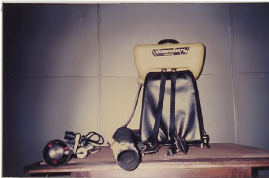
PLATE 3. Standard mistblower (50cc Wambo GmbH)
