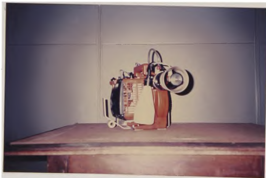
PLATE 4. Adapted Solo (GmbH) mistblower to provide a straight air jet.
