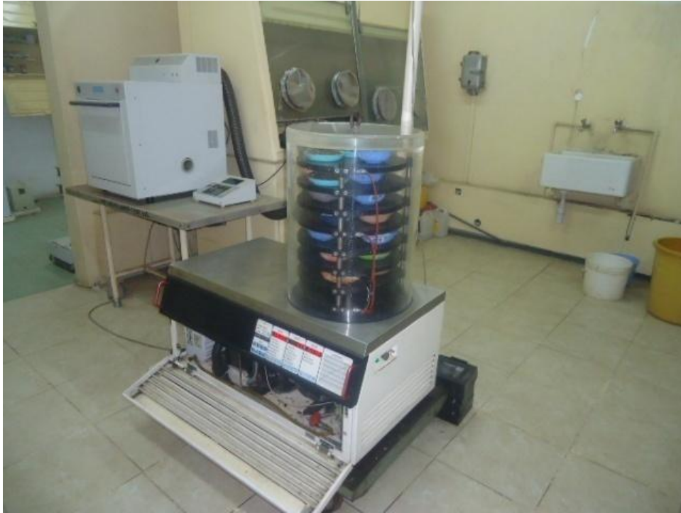
Plate 3.7: Freeze drying of plants samples
