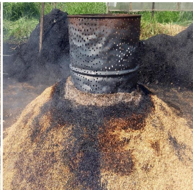
Plate 3.7 Charring heaped rice husk around barrel.
