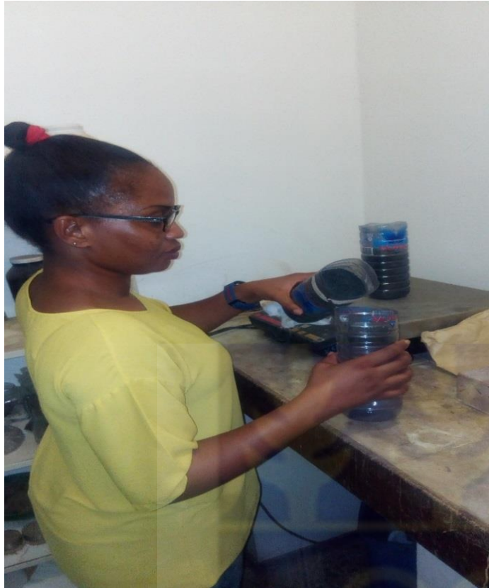
Figure A9 Weighing biochar and activated carbon for waste water filtration experiment.
