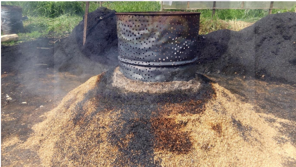
Figure A5 Biochar preparation (pyrolysis).
