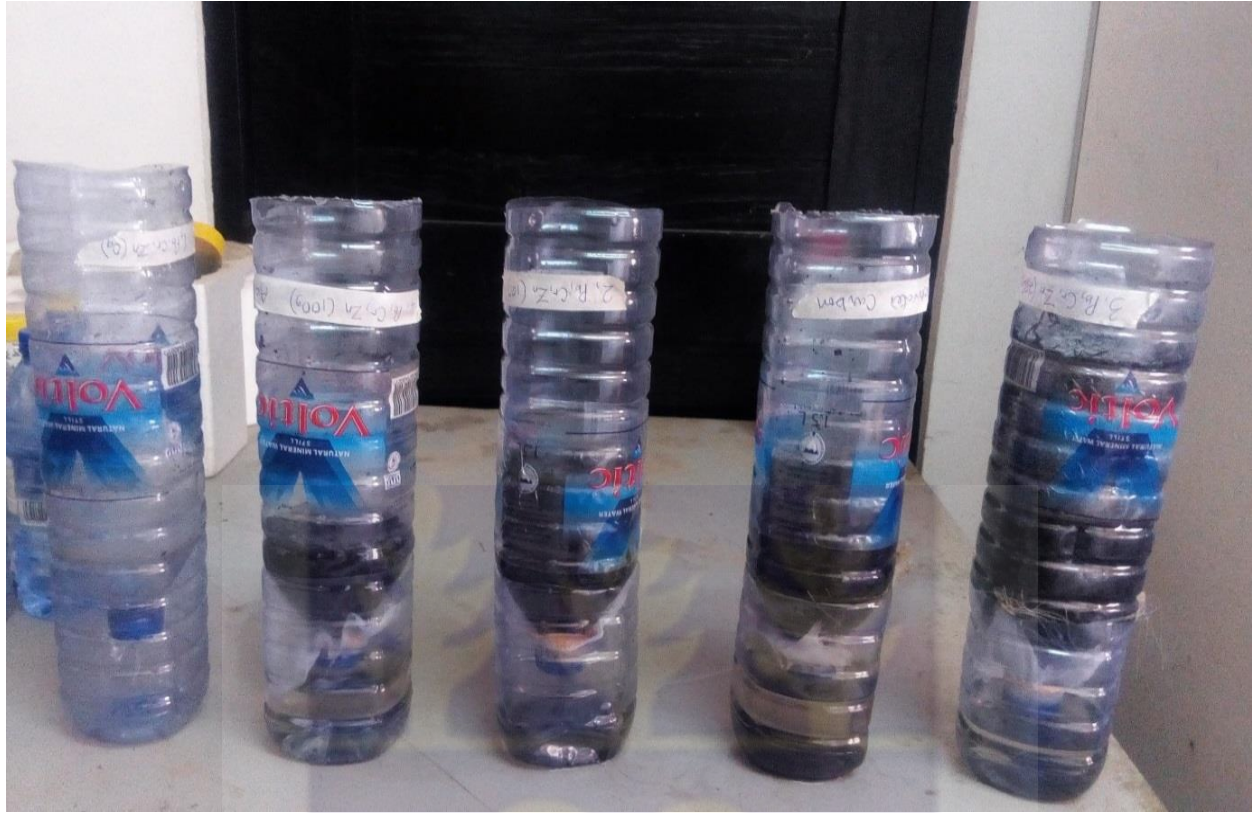
Plate 3.3 Set-up for waste water treatment (filtration) using biochar and activated carbon.
