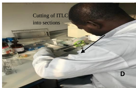
Fig.3.12D. Cutting of ITLC strip into sections to count
