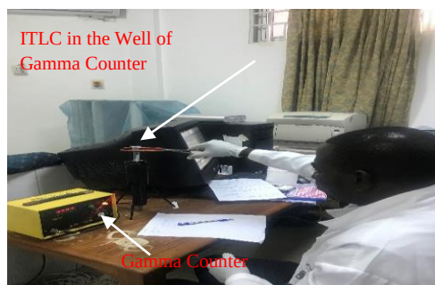
Fig.3.13 Radioactivity distribution counting in the ITLC sections.
