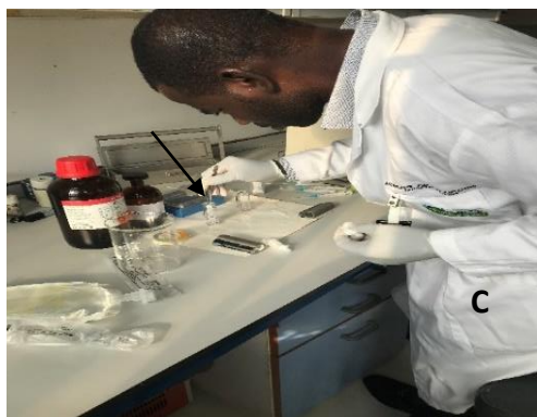
Fig.3.12C. Removal of ITLC strip from acetone chamber
