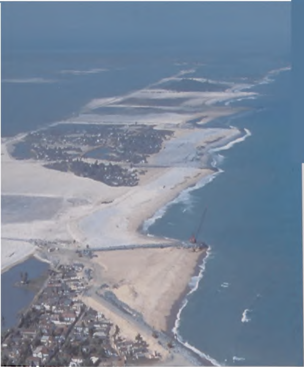
Figure 4.16 Aerial photograph of Keta showing part of the dredged channel, road, revetment, reclaimed area and the township. Photo by Great Lake Dry & Dock (GLDD).
