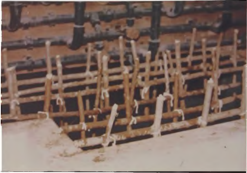
PLATE 7: Large concrete tank containing water, water plants, snails and Bamboo cylinders with test materials, under simulated natural conditions
