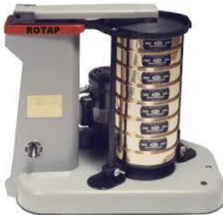
Plate 3. 2: A Rotap machine with 7 sieves
