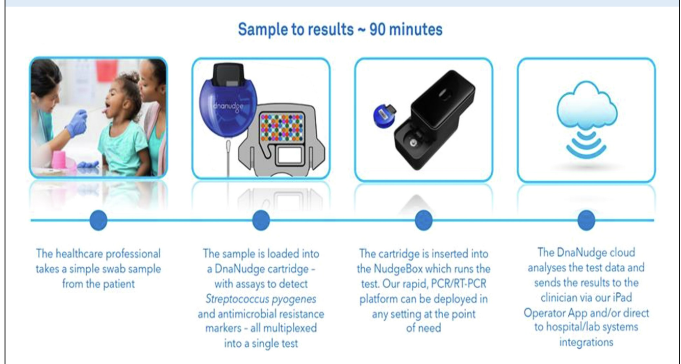
FIGURE 3 DNA Nudge Box Rapid Point of Care Device Demonstrating the Test Flow of the Strep a group A Streptococcus Test Screening, With Results in 90 minutes which Include Antimicrobial Resistance Targets
