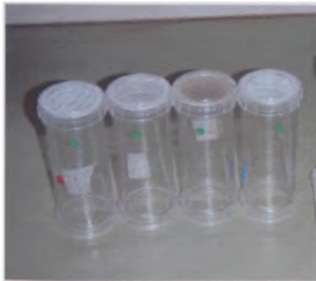
Figure 3.6: Bioassay experiment set set-up; a) Exposure tubes with insecticide impregnated papers (b) Holding tubes.
