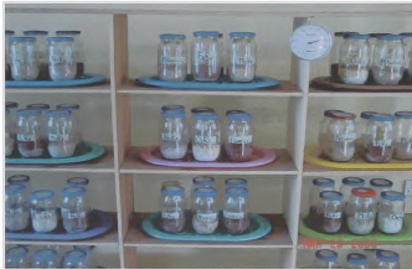
Plate 4: Experimental set up for weight loss determination without much compaction
