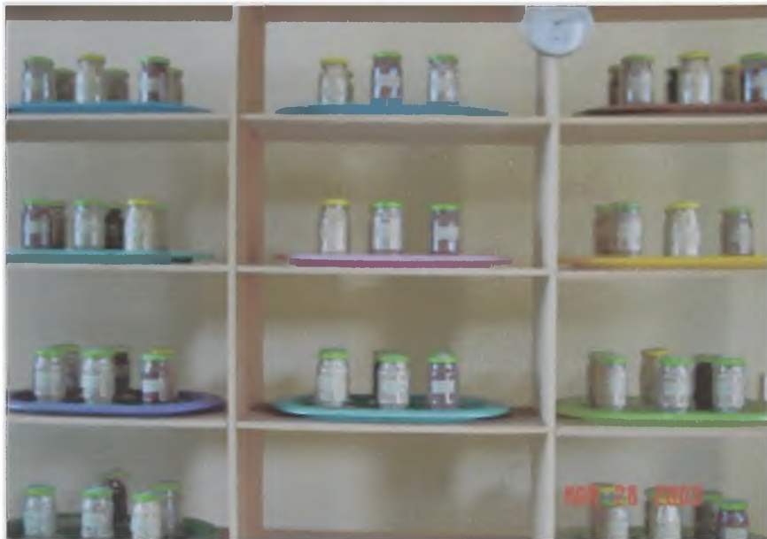
Plate 5: Experimental set up for weight loss determination with some level of compaction
