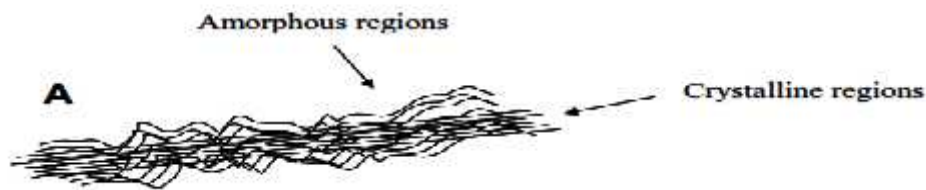
Figure 2.2: Crystalline cellulose is in the core of the microfibril, and it is surrounded by amorphous substrate.
