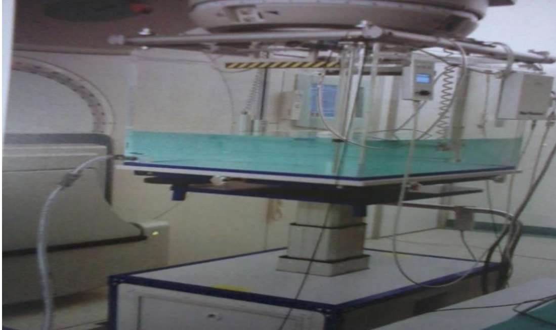
Plate 3.7 A pictorial view of the set-up for measuring TMR when the phantom was filled with 10 cm of distilled water
